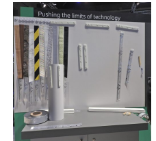
Ericsson "stripe" antennas Massive MIMO
